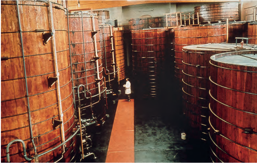
Figure 34 A glance into the vinegar plant of the company “Essig Kuehne KG” in Hamburg (Germany). The huge wooden reactors are made of oak. (Courtesy of the company.)
